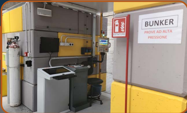
Bunker suitable for High Pressure Gas Tests: up to 15.000 PSI
